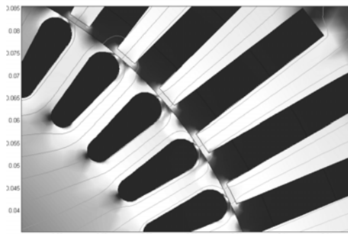
Fig. 3. Field distribution for the 2ЭKB3.5-210 type IM at rated condition
