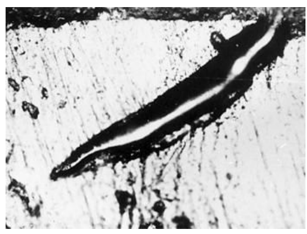
Fig. 3. Polished microsections of oil-coal granules with the penetration of oil into the coal substance.
