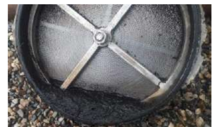
Fig E. Flame arrester (before and after using the port)
