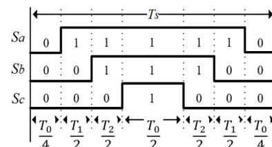
Fig. 10. Switching pulses waveform for the first 60°-sector
