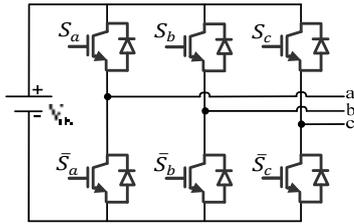
Fig. 1. Schematic diagram of a two-level VSI
