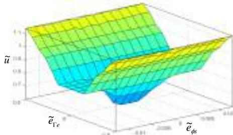
Fig. 8. Control surface of the fuzzy logic estimator
