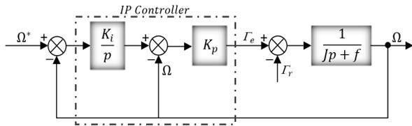
Fig. 4. Speed control loop with IP regulator
