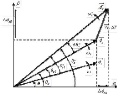
Fig. 12. Direct control of the stator flux vector
