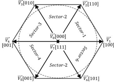
Fig. 2. Illustration of VSI state vectors in the  $\alpha$ - $\beta$  plane
