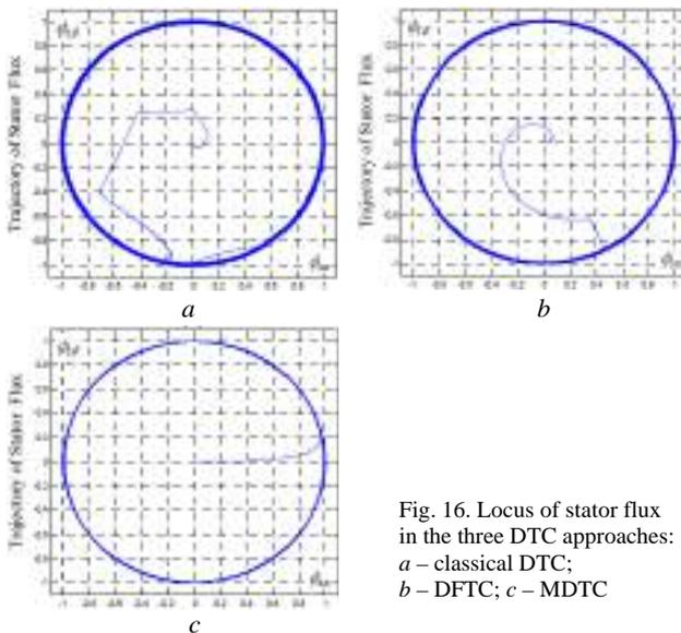
Fig. 16. Locus of stator flux in the three DTC approaches: *a* – classical DTC; *b* – DF-TC; *c* – MDTC
