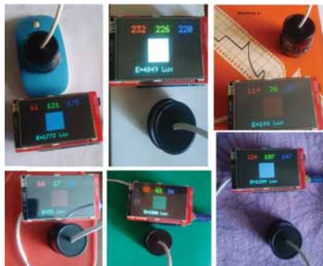
Figure 6. Examples of the work of the colorimeter: blue and red plastic; white, green and orange paper; magenta fabric
