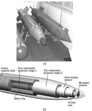
Fig. 2 Electromagnetic Bombs a - Russian GPS-guided KAB-500S type Electromagnetic Bomb (right); b - typical construction of an E-bomb
