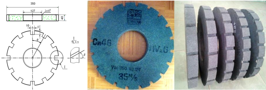
Figure 1 – Geometry parameter of segmented grinding wheel with angle \beta slot's width w and slot's depth b
