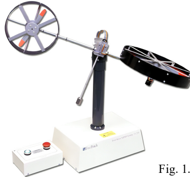
Fig. 1. The general view of the TRMS [23]
