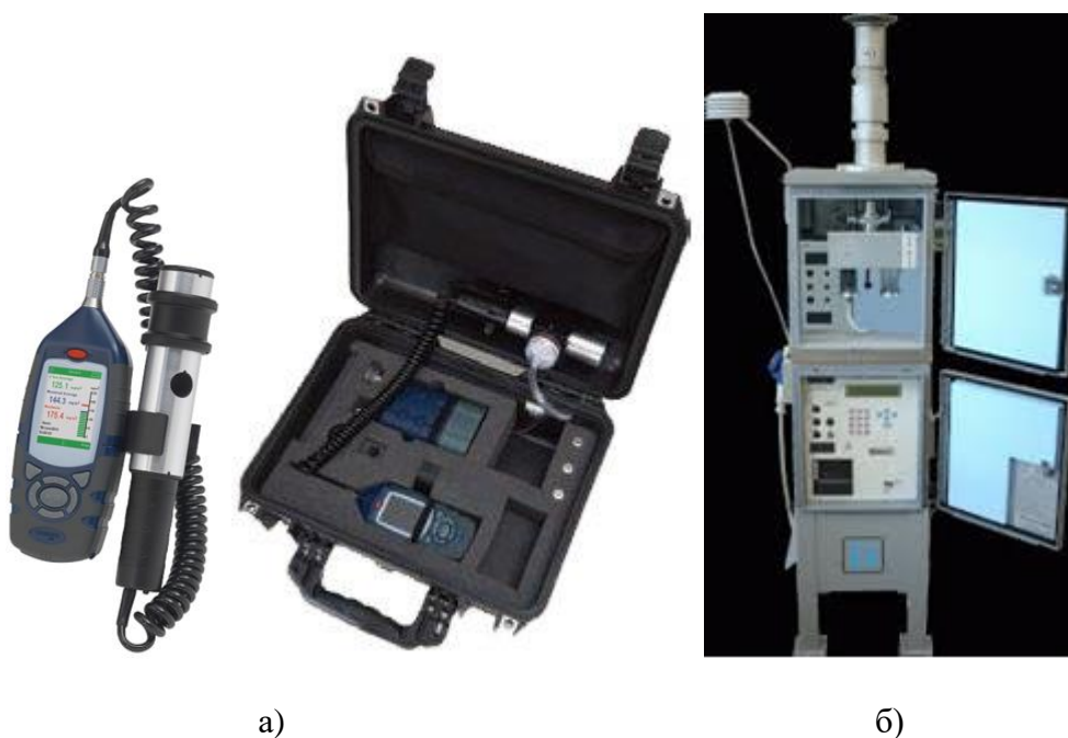
Figure 7 – Devices for recording aerosol particles in the air: a) dust analyzer CEL-712 Microdust Pro [25]; b) automatic model system ExplorerPlus (Zambelli, Italy) [26]
