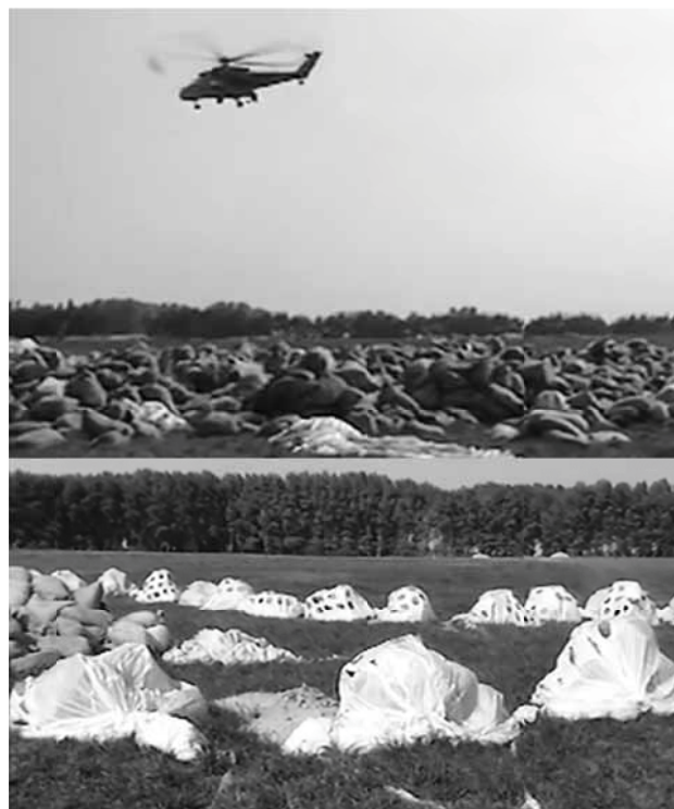
Figure 1. A helicopter over sandbags with dolomite and parachutes with boric acid and liquid rubber [3]
