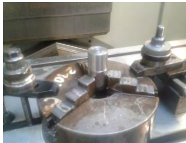
Figure 4 – Clamping of the machined specimen
