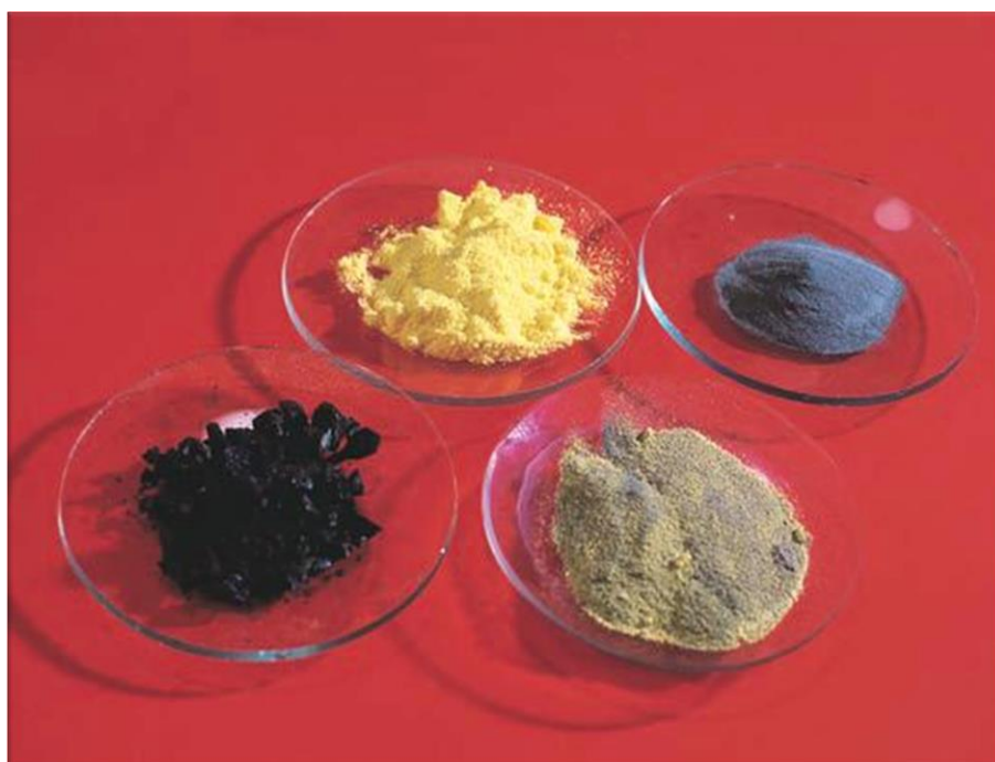
Figure 1.4. The elements sulfur and iron at the top of the photograph, and (below) black iron (II) sulfide on the left and a mixture of the two elements on the right.
