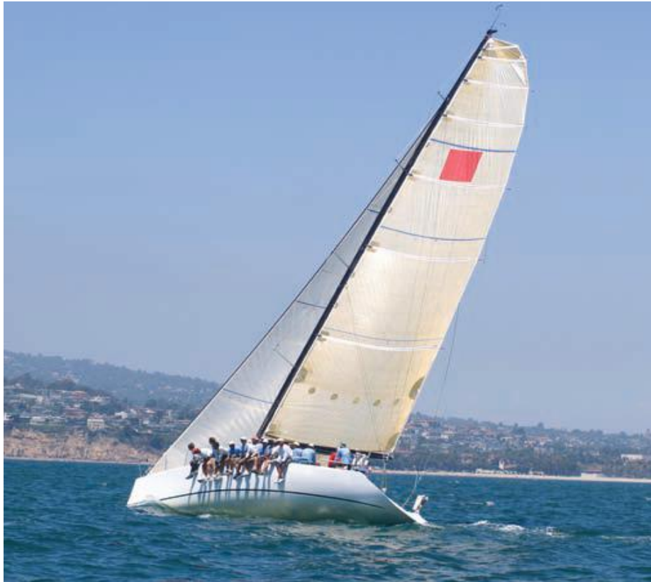
Figure 1.7. The glass-reinforced plastic used to make boats like this is a composite material.
