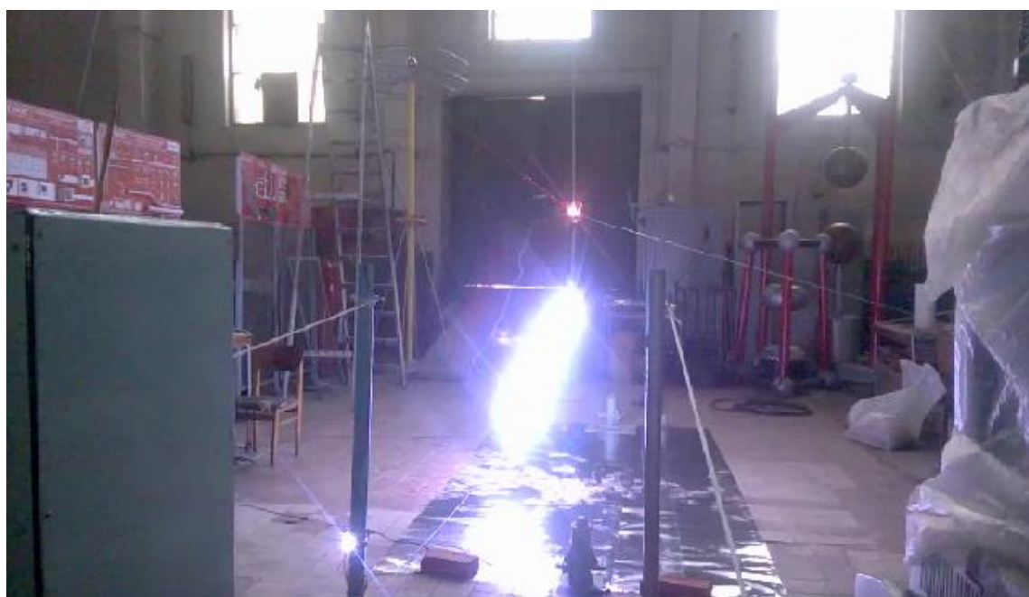
Figure 3.4 is a photograph of damage to an uninsulated wire on a large-scale model during the first series of experiments
