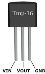
Figure 6.3 – TMP36 Temperature Sensor
