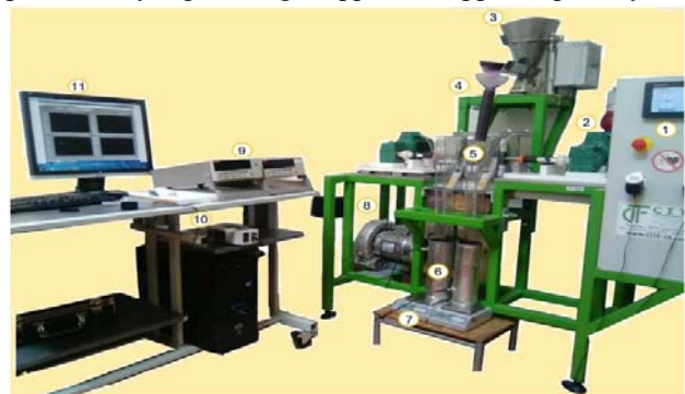
Fig. 1. Tribo-aero-electrostatic separator with two rotating disks: 1 – control panel; 2 – variable speed DC motors; 3 –vibrating feeder; 4 – cylindrical feeder; 5 – separation chamber with two rotating disk electrodes; 6 – Faraday cages; 7 – balances; 8 – blower; 9 – electrometers (Keithley 6514); 10 – portable colorimeter NH310; 11 – computer [7]
