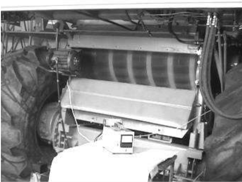
Fig. 9 – Location of DB-2K device and electric motor while balancing
