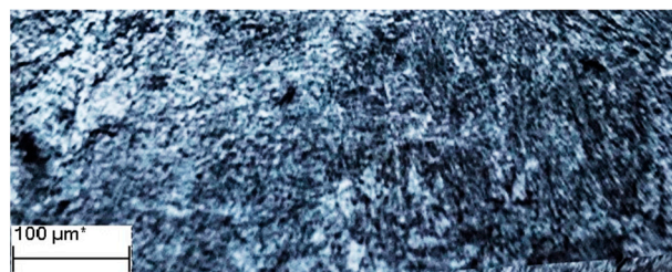
Figure 4. The structure of the base metal of the welded joint from the steel 25H2NMFA. \times 400 . *—mkm.
