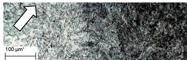
Figure 10. The fusion area (indicated by the arrow) of the HAZ of the welded joint, Template 3 (see Figure 11). \times 400 . *—mkm.
