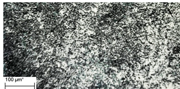
Figure 11. Structure of the overheating section, template 2 (Figure 7). \times 400 . *—mkm.
