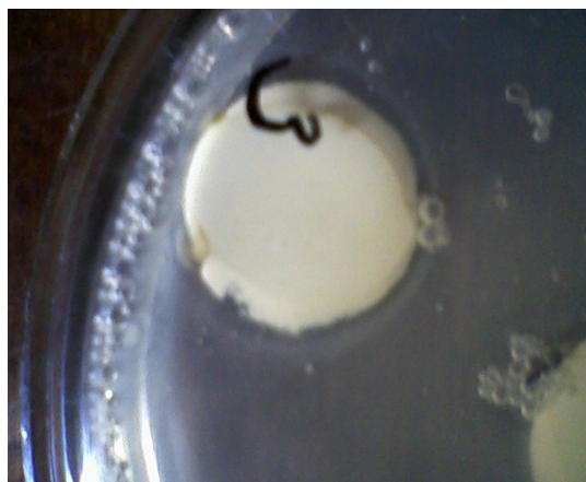
Figure 5. Zone of growth inhibition (dark areas) of Candida albicans around KF-11 specimen with \text{AgNO}_3 at inoculant density of 10^7 cells/cm 3
