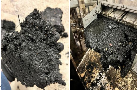
Figure 1 – Photo of dehydrated sludge after roller press
